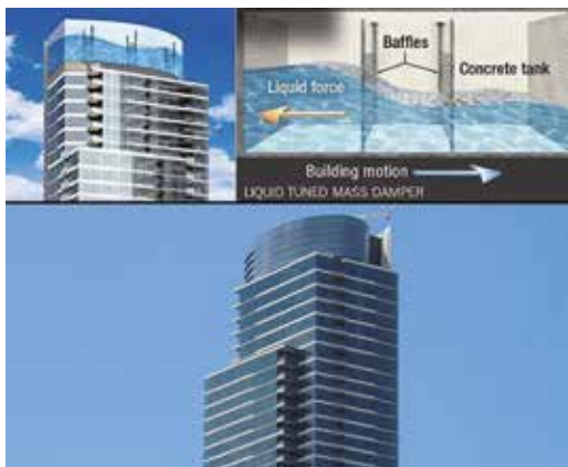
Figura 10. Sistema Tuned Mass Dampers: schema della Taipei 101 Tower in Taiwan (fonte: https://www.youtube.com/watch?v=1c2-ut_-7z4 )
